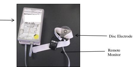
Figure 1: GED Electrical Stimulus Generation Module and Remote Monitor
